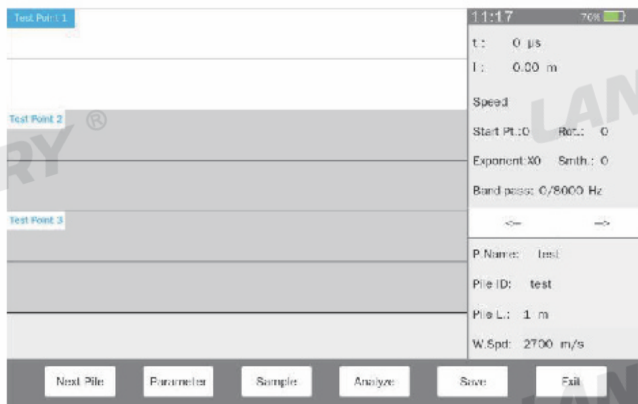
Figure 4-6 Pile Testing Interface
